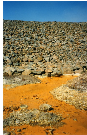
Mine effluent discharging from the bottom of a waste rock pile
